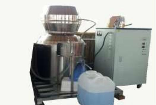
An electric distillation unit consisting of a large stainless steel boiler on a stand, connected to a condenser and a collection vessel. A control panel with a digital display and buttons is visible on the right side. |
