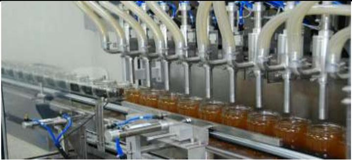
A photograph of an automatic filling machine in operation. The machine features multiple filling heads with white tubes, positioned over a conveyor belt. The conveyor belt is moving several glass bottles filled with a golden-brown liquid. The machine is stainless steel and has a clean, industrial appearance.         |
