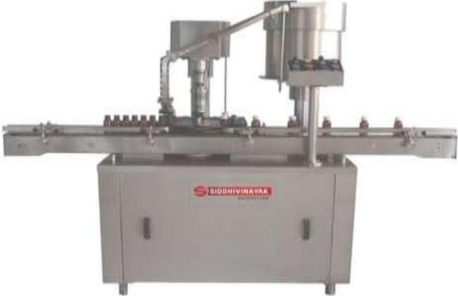
A photograph of an automatic screw capping machine. The machine is made of stainless steel and has a boxy, industrial design. It features a central mechanism with two large, vertical screw heads. The machine is mounted on a base with two doors and handles. The brand name "BIOBHIVANAK" is visible on the front panel. |
