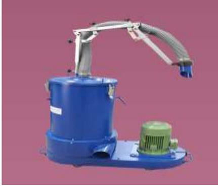
A blue industrial dust collector with a green motor and a flexible extraction arm, used for capturing dust during grinding. |
